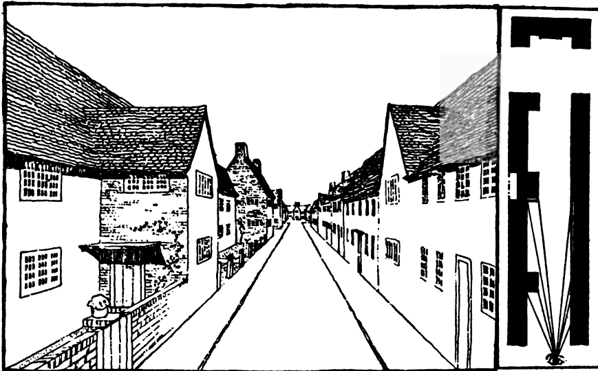
Illus. 191.—Plan and sketch of street showing on one side the uninteresting vanishing perspective of the unbroken building line, and on the other the more picturesque result of breaks.
